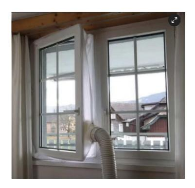
The room's heat is removed from the AC via a hose. It must go out through a window or patio door. To prevent heat from outside and small insects from entering, you should install a window seal. They are available in different designs.
